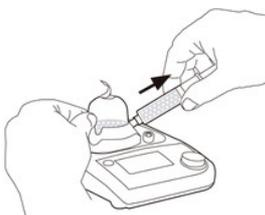
Keep the capsule on the stirrer, and while it continues to stir at low speed, carefully aspirate the foam at a rate of not more than 1 mL per second, up to a maximum total of 1 mL of foam.
