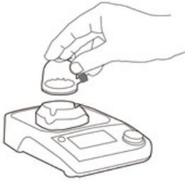
Remove the VARIXIO® Pod Air from its bag and put it in the docking site on the VARIXIO® Pro Mag stirrer in the left- or right-handed position, as appropriate.
