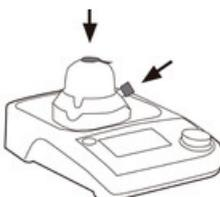
Close the Luer cap. The remaining foam can be kept at low-speed stirring for later use for up to 15 minutes.
