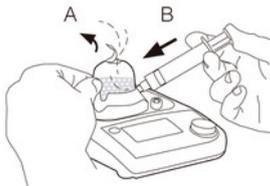
Before aspirating the foam, open the top seal (A) and press down the syringe (B) to empty it of any air it may contain.
