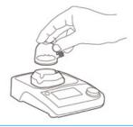
Remove the VARIXIO® Pod Air from its bag and put it in the docking site on the VARIXIO® Pro Mag stirrer in the left-or right-handed position, as appropriate.
